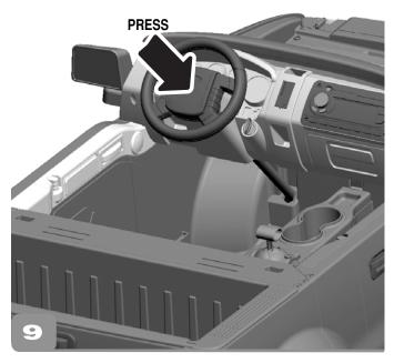
• Press the steering wheel down to "snap" into place.
